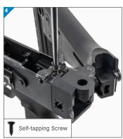
The 1/2 inch Self-tapping Screw is included to secure the folding adaptor hinge base to the inside of the firearm. Ensure the adaptor stays flush against the receiver as this will fix your stock. (Optional: Drill a 1/16 inch hole into the folding adaptor. Do not exceed a 1/2 inch depth.)
