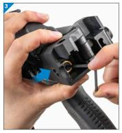
Hold the folding adaptor flush in place to the receiver. Use the 3 mm Hex Key to tighten the inner screw CLOCKWISE. Tighten until the screw no longer spins. Do not forcefully overtighten or it will create a gap.
