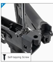
The 1/2 inch Self-tapping Screw is included to secure the folding adaptor hinge base to the inside of the firearm. Ensure the adaptor stays flush against the receiver as this will fix your stock. (Optional: Drill a 1/16 inch hole into the folding adaptor. Do not exceed a 1/2 inch depth.)
