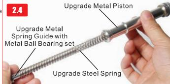
**Tip:** Apply high quality grease on the Rubber Ring of the Upgrade Metal Piston could reduce the resisting force and smooth cocking operation.
