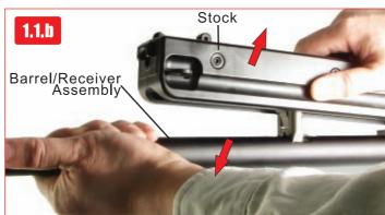
Step 1.1: Remove the magazine. Dry shoot the gun at a safe direction to make sure there is no BB left in the gun, and the gun is uncocked. Remove the two screws (Fig. 1.1.a) and separate the Barrel/Receiver Assembly from the Stock (Fig. 1.1.b). (If upgrading a new Shadow Ops that has not been assembled out of The box, bypass this step.)
