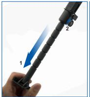
Pull down the foot pad to increase the length of the leg extension. Note that the leg extension is under spring tension as it is designed to automatically retract. The leg extension is keyed and once at the desired length is secured in place by turning back the locking thumb wheel clockwise until it stops.
