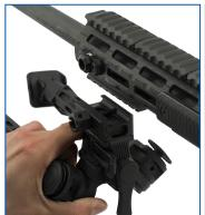
1. Position the bipod so that the tilt tension adjustment lever is facing away from the muzzle.
