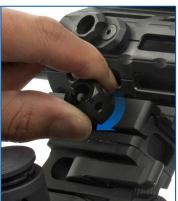
3. Retighten the side locking plate nut by turning it clockwise until snug or to 50in-lb using a torque wrench equipped with a 5/8" socket.
