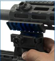
2. Loosen the side locking plate nut by turning it counterclockwise. Loosen it enough for the mounting interface to seat evenly onto your firearm's MIL-STD-1913 Picatinny rail and with its squared recoil stop fitting into the rail slot.
