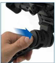
1. Push down the posi-lock push button until you feel its locking lugs disengage, allowing you to rotate the bipod leg to another position.
