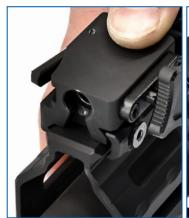
5. The QD mounting base should be positioned on the 12 O'clock rail and as far forward on the rail as possible towards the muzzle.
