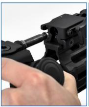
7. Insert the bipod back into the QD mounting base, making sure the base's locking lever reengages.
