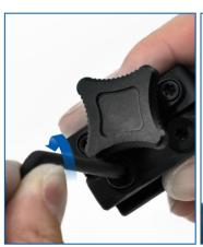
3. Loosen the QD mounting base's side locking plate by turning its screws counterclockwise with the included tool.
