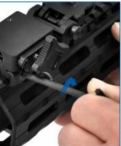
6. Retighten the side locking plate by turning its screws clockwise until tightened. Recommended torque value is 35 in.lb.
