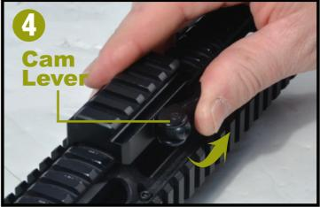
4. The optimal tension is achieved when the side plate first makes contact with the rail while the Cam Lever still has enough travel left for you to securely snap into its locking position. Once you achieve the optimal tension, push the Cam Lever all the way to the right for a positive lock onto the rail. You may repeat Step 3 and 4 if needed to find the best clamping tension and locking position for your QD adaptor on the rail.
