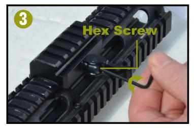
3. Use the included Allen wrench to adjust the Hex Screw at the side of the cam for proper tension and fit against the rail. Adjust clockwise to increase the tension and reduce the clamping width. Adjust counter-clockwise to decrease the tension and increase the clamping width.
