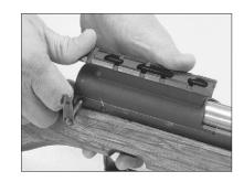
5. Align the receiver cover locking pin with the pin hole on the rear of the scope mount.
