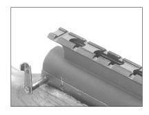
7. Test drive the bolt carrier and check the movement under the receiver cover mount to ensure that there is no obstruction to the bolt operation. Your scope mount is now fully seated and fitted into receiver, and is ready for ring and scope installation.
