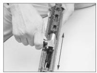
9. Put the rifle to your shoulder in your natural shooting position and adjust the scope eye relief until you achieve a full field of view. When you find the ideal eye relief, rotate the scope so that the crosshairs are vertical and perpendicular to the rifle.
