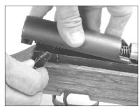
3. Place the mount in a vise with padded jaws for protection. Bend one of the front prongs very slightly. This will allow a snug fit of the cover both vertically and horizontally, and improve shooting accuracy.
