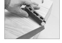
4. Slide the scope mount onto receiver. Press it forward and down until the front prongs are inserted into the receiver completely.
