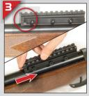
Hold the mount in front of the dove tail. Align the rear of the mount with the front end of the dovetail rail. Slide the mount backward on the dovetail rail until the recoil stop shoulder of the mount contacts the front end of the dovetail rail.
