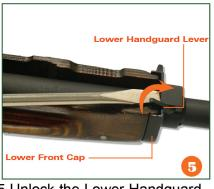
5.Unlock the Lower Handguard Lever on the Lower Front Cap.
