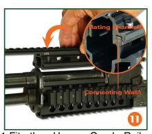
11.Fit the Upper Quad Rail System onto the gas tube. Make sure the 2 Connecting Walls of the Lower Quad Rail System fit into the 2 Mating Channels of the Upper Quad Rail System.
