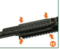
12.Evenly tighten all 4 screws to securely connect lower and upper quad-rails. Replace the bolt, the bolt carrier/gas piston, the action spring, the retaining rod and the receiver cover.
