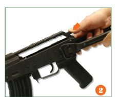
2. Push the Release Button again to lift and remove the action spring and the retaining rod.
