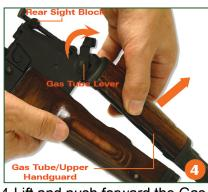
4. Lift and push forward the Gas Tube Lever next to the Rear Sight Block and take out the Gas Tube/Upper Handguard Assembly.
