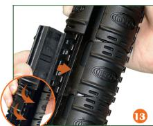
13.Align the Cross Bar of the Rubber Rail Guard to a desired rail slot on a rail. Extend the Rubber Rail Guard to horizontally situate the Cross Bar over the rail slot. Push the whole piece to click into the rail for a tight fit.
