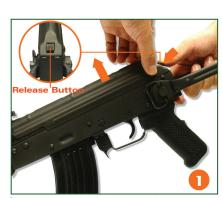
Press the Release Button to lift and remove the receive cover.
