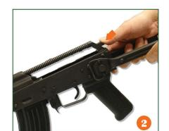
2. Push the Release Button again to lift and remove the action spring and the retaining rod.
