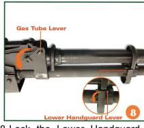
8.Lock the Lower Handguard Lever on the Lower Front Cap. Replace the gas tube and lock it down by turning the Gas Tube Lever back and downward.
