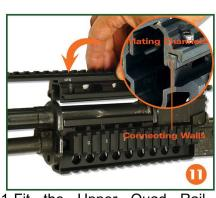
11.Fit the Upper Quad Rail System onto the gas tube. Make sure the 2 Connecting Walls of the Lower Quad Rail System fit into the 2 Mating Channels of the Upper Quad Rail System.
