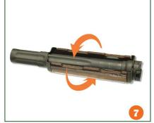
7.Twist the Upper Handguard to separate the handguard from the gas tube.
