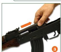
3. Remove the bolt and the bolt carrier, including the gas piston attached to the bolt carrier.
