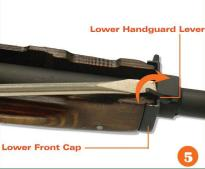
5. Unlock the Lower Handguard Lever on the Lower Front Cap.
