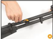
4. Place the 2 Barrel Spacers between the barrel and the gas tube at mid section as shown in . Tighten the 2 screws to lock the spacers firmly. Barrel Spacers must be installed to prevent over tightening of the top/bottom covers and to allow for normal operation of the piston.
