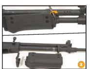
Turn forward the Locking Lever on the Front Holder (Cap) of the Handguard with a screwdriver. Move the Front Holder (Cap) forward to remove the spring, handguard, and the Rear Holder (Cap).
