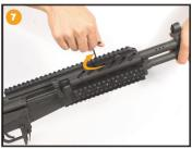
7. Evenly tighten all six screws to securely lock the top and bottom
