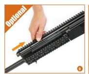
9. Based on your need, select either the longer or shorter Top Cover, and slide it onto the Middle Cover, with the two connecting walls of the Middle Cover. Fitting with the mating channels of the Top Cover.
