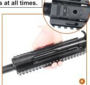
4. Fit the Bottom Cover onto the barrel and make sure the fit is even and level. Make sure the through hole at the front end of the bottom rail is aligned well with the screw hole under the front sight block.
