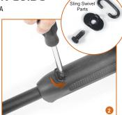
2. Disassemble the front sling swivel at the front end of the bottom polymer handguard with a screwdriver, and separate the screw, oval plate and loop.
