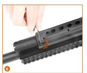
6. Evenly tighten the four M4 screws with the provided Allen wrench to securely lock the middle and bottom covers
