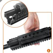
5. Fit the Middle Cover onto the gas tube. Make sure the two connecting walls of the Bottom Cover fit into the two mating channels of the Middle Cover.
