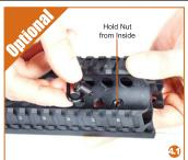
4.1 (Optional Step) - Pre-assemble screw, cylinder and loop. Hold and position the assembly in one hand onto a selected ventilation hole. Position and hold the nut on the opposite side of the ventilation hole.
