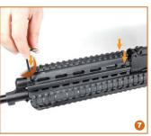
7. Evenly tighten all 4 screws with the provided Allen wrench to securely lock the top and bottom covers.
