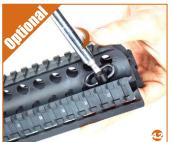
4.2 (Optional Step) – Use a screw driver to tighten the Sling Swivel to the bottom metal handguard.
