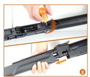
2. Remove the locking screw at bottom of the receiver with a screwdriver. Slide the polymer handquard forward, and remove it away from the barrel.
