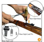
Punch the Rear Sight Leaf Pin out with a hammer and a proper puncher. Take off the Rear Sight Leaf and the Leaf Spring.
