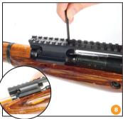
Align the screw holes on the top mount with corresponding holes on rectangular steel base, and tighten the two M5 locking screws firmly.
