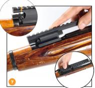
Position the top mount with tail end toward to receiver, and place it onto the rectangular steel base and align so that the bottom slot of the top mount fully engaged with the cross bar on the rectangular steel base.
