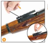
Tighten the two M3 side screws to lock rectangular steel base with the firearm rear sight base, and tighten the two M5 top locking screws to lock the rectangular steel base with the steel spacer firmly.
