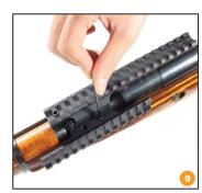
Install the side rails with the provided M4 locking screws.
