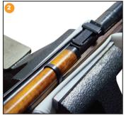
Place the rifle in a vise with padded jaws to protect and hold the firearm firmly.
