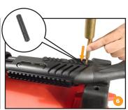
Turn over the gun. Tap on the right end of the Rear Trigger Retaining Pin and remove it from the left side of the gun.
