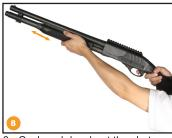
Cock and dry shoot the shotgun to make sure it is in good working order. Now you can install rings and scope on the top rail of the mount.
