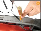
Take out the Front Trigger Retaining Pin with a proper brass drift punch and a hammer.
