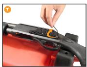
Set the gun with left side up again. Replace and tighten firmly the larger screw supplied with the mount from the left side.
