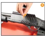
Replace and tighten firmly the smaller screw supplied with the mount from the left side with provided Allen wrench.
