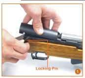
Locate the receiver cover of your rifle. Pull out the locking pin. Carefully and gently lift and remove the existing receiver cover. Do not pull too quickly which may result in sudden release of the bolt operating spring.
