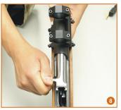
8. Test drive the bolt carrier and check its movement under the receiver cover mount to ensure that there is no interference to the bolt operation. If there is any interference, DO NOT use until it is resolved. Your scope mount is now fully seated and fitted into receiver, and is ready for scope installation.
