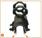
4. Place the mount in a vise with padded jaws for protection. Bend one of the front prongs very slightly. This will allow a snug fit of the cover both vertically and horizontally, and improve shooting accuracy.
