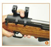
5. Slide the scope mount onto receiver. Press it forward and down until the front prongs are inserted into the receiver completely.
