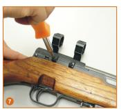
7. Tighten the 4 Set Screws and the nuts.
