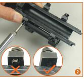
Loosen the 4 Set Screws on the mount with a flat screw driver. Make sure they are loosened enough so that they do not stick out through the holes.
