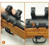
6. Align the Locking Pin with the pin hole at the rear of the scope mount. Drive the locking pin back into receiver using your finger or gently tapping with a rubber mallet until the pin is flush with the receiver surface at the opposite end. Then, turn the locking pin handle forward to secure a tight lock. Due to different rifle variants, the rear pin hole area may need minor filing for best fit.
