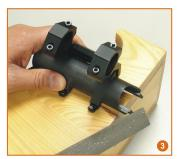
3. The receover cover mount is made intentionally longer than the original receiver cover. Gently file the front two prongs of the mount if they are too long for your firearm. DO NOT over file. Maintain prong angle to ensure a good snug fit.
