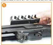
Place and hold the shot shell carrier on the left side of the mount's screw holes with that of the carrier's. The carrier should be orientated so that it overlaps the receiver only and not where the stock meets the receiver
