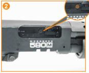
With the pump arm rearward, remove the OEM ejector screw from inside the receiver using a flathead screwdriver. Partially install our flathead ejector screw until the face of the screw is flush with the outside of the receiver.
