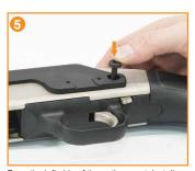
From the left side of the optic mount, install our Torx receiver pin. Lightly tapping the pin through may be required. Insert the squared nut into the squared cutout on the right side of the mount and hold it in place.
