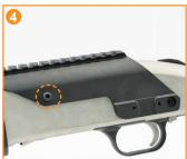
Screw the flathead ejector screw the remainder of the way from the inside until it is tight against the receiver. Install and hand tighten our Torx ejector cap onto the ejector screw from the outside.
