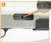
With the pump arm rearward, remove the OEM ejector screw from inside the receiver using a flathead screwdriver. Partially install our flathead ejector screw until the face of the screw is flush with the outside of the receiver.
