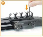
Insert the included Hex screws and tighten using the included tool. Recommended torque value is 15 In-lbs.
