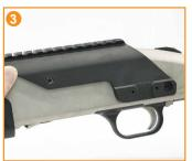
Place the optic mount on top of the receiver and align the optic mount's receiver pin hole and ejector screw hole with that of the receiver.
