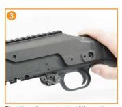
Place the optic mount on top of the receiver and align the optic mount's receiver pin hole and ejector screw hole with that of the receiver.
