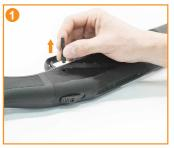
With the safety on, remove the OEM receiver pin just above the action release tab by lightly tapping the pin out with a proper hammer and punch.
