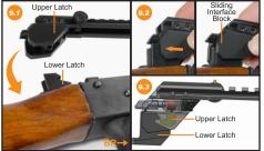
9.Lower the Sight Rail onto the Base Block (Fig. 9.1). Pull the Sliding Interface Block rearward to obtain complete engagement between the Upper Latch in the Sliding Interface Block and the Lower Latch in the Base Block (Fig. 9.3). A 20mm forward-backward adjustment range is provided by the Sliding Interface Block to allow secure mount installation on different AK variants.
