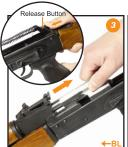
3. Push the Release Button to remove the action spring and then remove the bolt carrier group.
