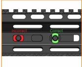
If the T-Nuts are spaced with too much gap they will rotate freely when trying to tighten. Alternately, if the T-Nuts are not spaced with enough gap they will not rotate at all. Observe the T-Nut during the installation process to be certain that they have rotated to their correct position as shown.
