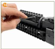
Evenly tighten the four locking screws using a cross torque pattern with the included tool while making sure the upper and lower portions of the handguard are kept level. Recommended torque value is 20 in-lbs.
