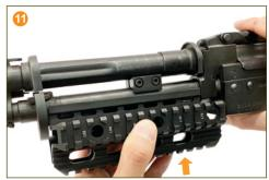
Install the lower portion of our handguard and test for fitment. Reposition the barrel spacer if necessary for the handguard to seat properly against the barrel. If the fitment is loose proceed to step 13. If the fitment is tight and secure, proceed to step 14.
