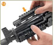
Install the top portion of our handguard over the gas tube and align the screw holes with that of the lower portion of the quad rail. The top portion should not interfere with the barrel spacer and should seat evenly on top of the lower portion.
