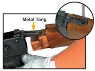
3. Unscrew the 2 buttstock screws and remove the buttstock.
