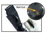
5. Align the set screw on the adaptor with the Slot Cut on the buffer tube. (Loosen the adaptor if needed.) Tighten down the set screw to securely lock the adaptor onto the tube.
