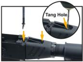
8. Once the adaptor is properly installed, use the 2 tang holes on the receiver as the guide to drill two 1/8" holes into the stock adaptor through the tang holes. Insert the self-tapping screws provided with the adaptor. Gently tap and then tighten to complete installation.
