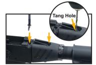
8. Once the adaptor is properly installed, use the 2 tang holes on the receiver as the guide to drill two 1/8" holes into the stock adaptor through the tang holes. Insert the self-tapping screws provided with the adaptor. Gently tap and then tighten to complete installation.
