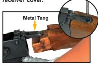
3. Unscrew the 2 buttstock screws and remove the buttstock.
